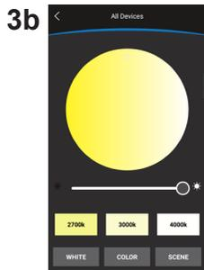
(3b) A long press from the home screen will bring up the control screen for changing the white color temperature of the lamps. There are 3 preset options for 2700K, 3000K and 4000K. A color wheel is also available for choosing other color temperatures. The slider in the middle of the screen will dim the light, sliding left will make the light dimmer, and sliding right will make the light brighter.
