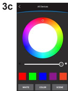
(3c) Clicking on the “COLOR” button at the bottom center of the page will bring up the control screen for changing the light to RGB colors. There are presets for Red, Green, Blue, Purple and Amber. A color wheel is also available for choosing other RGB colors. The slider in the middle of the screen will dim the light, sliding left will make the light dimmer, and sliding right will make the light brighter.
