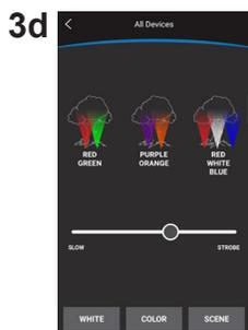
(3d) Clicking on the “SCENE” button at the bottom right corner of the page will bring up the control screen for changing the light to a preset scene. There are three preset options of Red+Green, Purple+Orange, and Red+White+Blue. The light will automatically cycle through each scenes preset colors. The slider in the middle of the screen will change the speed in which the colors cycle through the scene. Sliding left will slow down the cycle, and sliding right will speed up the cycle.
